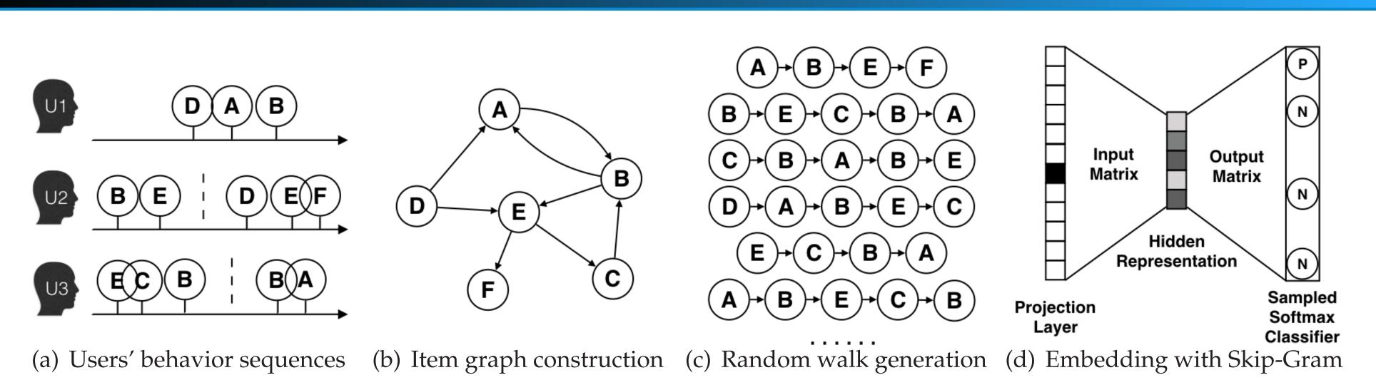
• Graph Construction: We construct item graph from users' behaviors and filter out invalid data and
